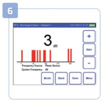
The discharge pattern screen displays where the PD is occurring on a mains cycle time base. Patterns can be compared to distinguish between PD and electrical noise as PD is synchronised to the mains cycle.
